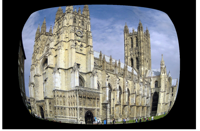
Fig. 8. Target distorted with the non-monotonic model f(r) = r - 0.5r^3 + 0.2r^5 + 0.5r^7 - 2r^9 (fold at r = 0.686 ). Undistorted content at r_{\text{in}} \leq r_{\text{fold}} is compressed into the disk of radius f(r_{\text{fold}}) = 0.523 ; content beyond the fold is non-invertible and is left black in place. Frame dimensions are preserved. The visible interior is well-structured, confirming that the hard-loss band is thin (4.9% of the image domain).
